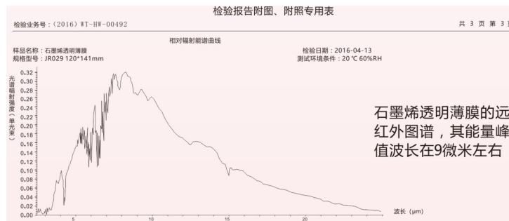
图1 石墨烯发热膜的红外线谱图 Fig.1 Infrared spectrum of graphene thermal film
